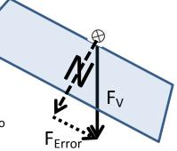
The component of the force we care about is  $F_{Error}$  – called that because this *is* the component of vertical magnetic force (the 'dip) that causes all of the turning and acceleration errors.
