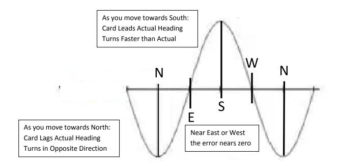
As noted previously – when turning through (or from, or even near) east or west the turn error moment arm goes to zero so the error goes to zero, as shown in the graph above. Turn error is greatest when near north or south and the error when near north is opposite of the error when near a southerly heading.
