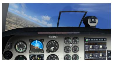
And one more thing that you need to remember. When you are looking at a whiskey compass you are viewing it from the 'back' – that is, if your aircraft is facing north the compass needle is attracted to the north (the far side of the compass itself) but you are seeing the 'south end' of the compass – even though it has a big 'N' on it, that is the side with the south end of the compass needle. So, when you are
